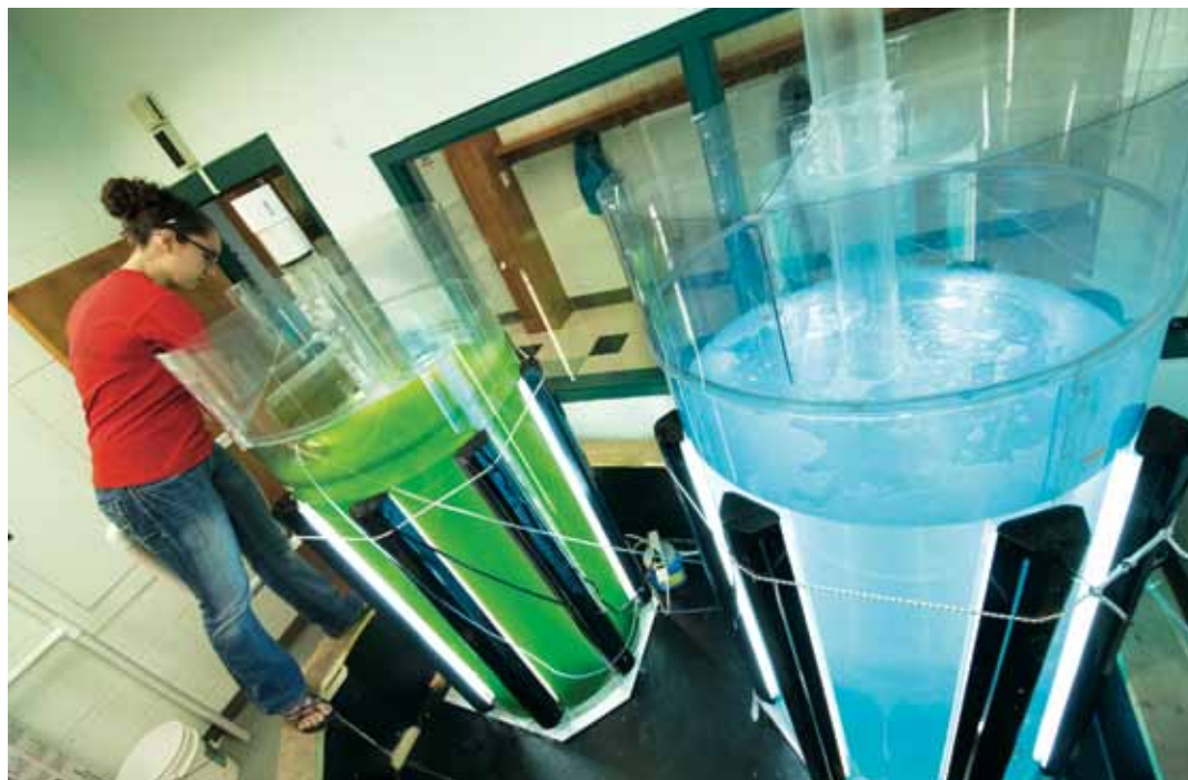
Photobioreactors: the blue tank contains nutrient only and the green tank has healthy live algae growth
