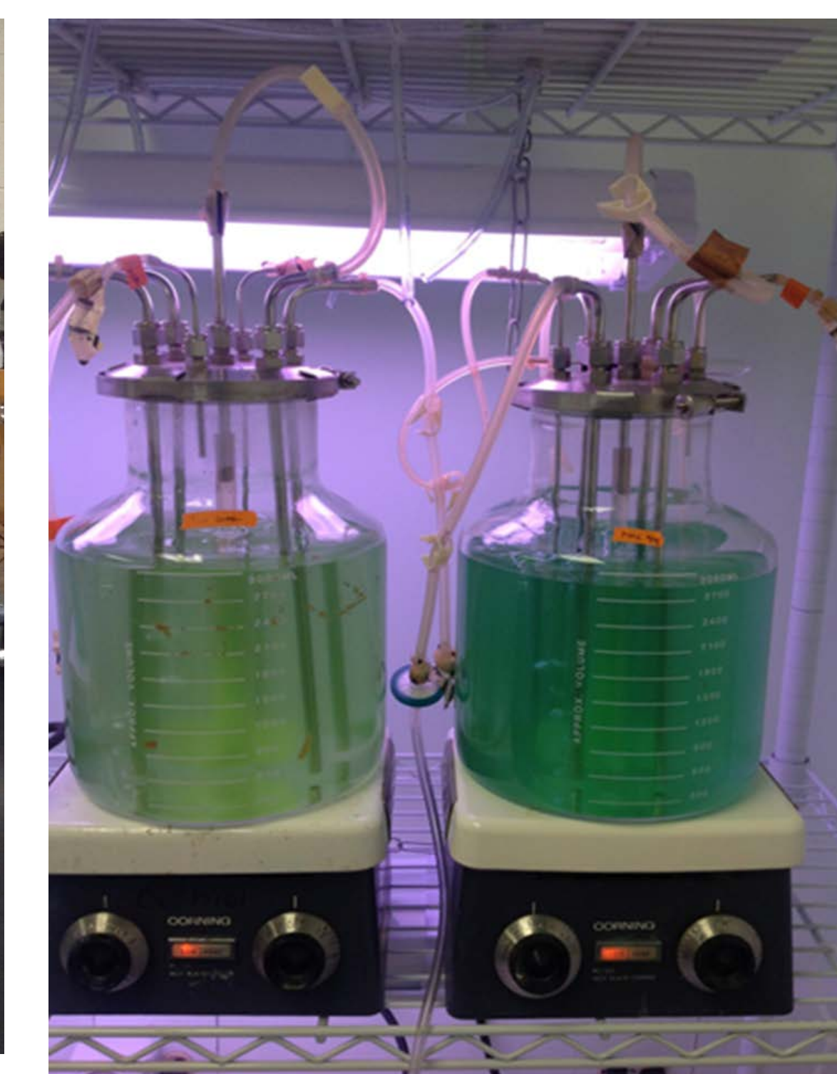
Figure 3: The 3L bioreactors were placed on magnetic stirrers to keep the algae suspended.
