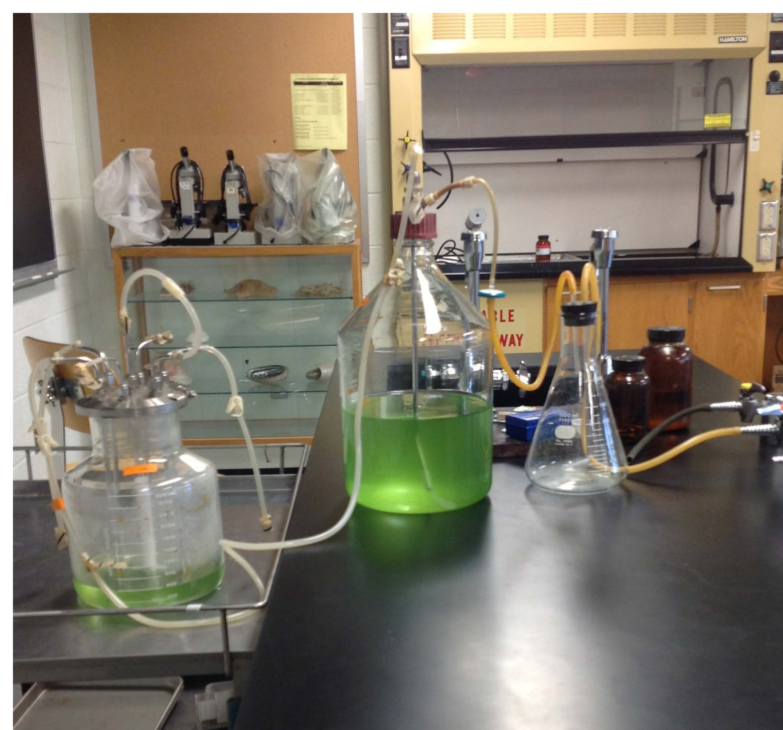
Figure 2: By blowing air from an air valve into the 5L bottle, we were able to force the liquid out of the 5L bottle and into the 3L bioreactor.
